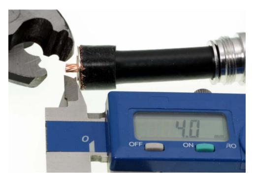
Our coax cable scissors cut the center conductor in a way that its stucture does not change. You can easily put the center pin onto the the cable.
