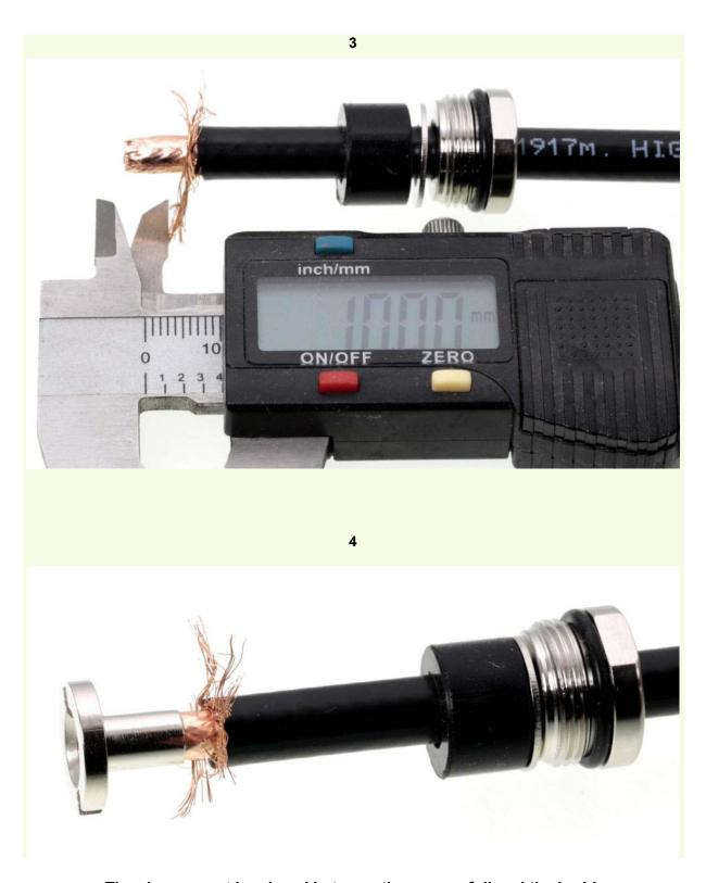
The clamp must be placed between the copper-foil and the braid.
