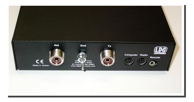
**ANT connector:** Connect the 50-ohm coax antenna feedline to this standard SO-239 connector.
