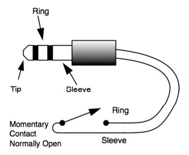
The remote switch may be mounted in any convenient location.
