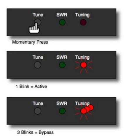
**Initiate a Memory Tune Cycle:** To initiate a memory tuning cycle using the front panel of the KT-100, you must first change the radio's mode to one of the continuous carrier modes, such as AM, CW, or FM. Press and hold the **Tune** button on the front of the KT-100 until the **Tuning LED** lights up. Key the transmitter and release the **Tune** button. A memory tuning cycle will begin. When tuning is complete, you may return to the operating mode previously set.
