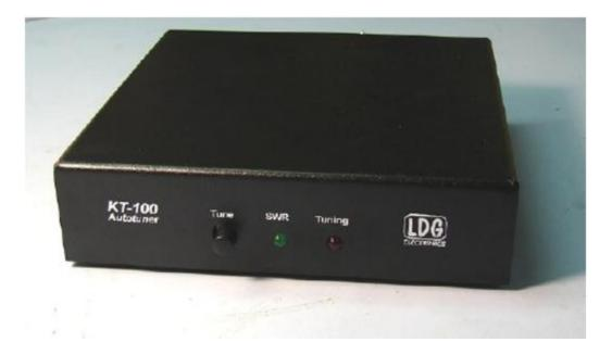
**Tune:** Initiates either a memory tune or a full tune, and also toggles the tuner between "active" and "bypass" modes.
