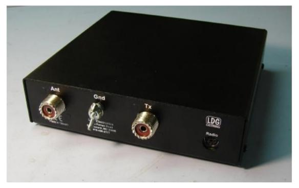
**ANT connector:** Connect the 50-ohm coax antenna feedline to this standard SO-239 connector.
