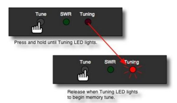
**Force a Full Tune Cycle:** Sometimes, if you are transmitting on a previously tuned frequency, but something has slightly changed in your antenna system (maybe the antenna was re-oriented, for example), performing a memory recall tune will find a stored match that is acceptable, but is not as optimal as could be. In this case, forcing a full tune will cause the KT-100 to seek a better match than the match already stored in memory for this frequency.
