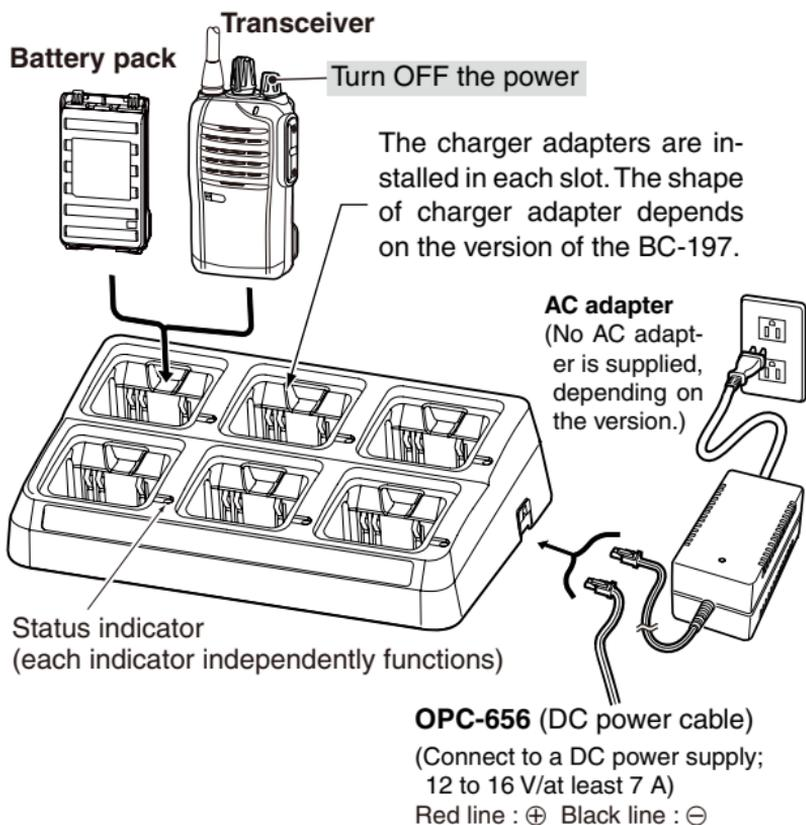
There are two types of BC-197 chargers for the transceiver; one is for Ni-MH batteries, and the other is for Li-ion batteries.
