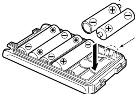
**Be careful!** The negative terminals of the battery case protrude from the body, so pay attention not to injure your fingers when inserting the batteries.
