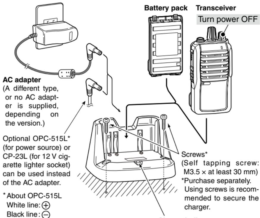
**CAUTION: NEVER** connect the OPC-515L to a power source using reverse polarity. This will ruin the battery charger.
