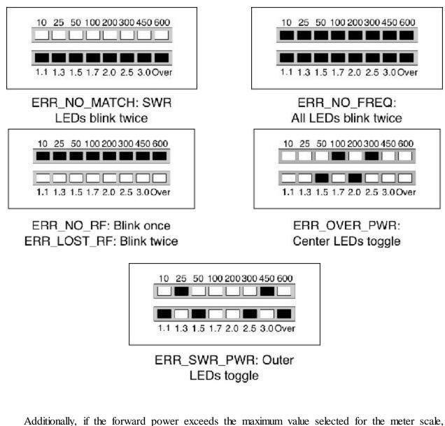
Additionally, if the forward power exceeds the maximum value selected for the meter scale, the PWR LEDs will blink an over-range condition. The four right-most LEDs of the PWR bargraph will cycle during over-range.
