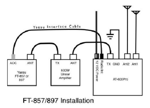
*Note: Optional Y-ACC cable has a red plug on the radio end of the cable, and a black plug on the tuner end.*
